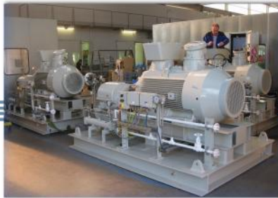
■ Variable frequency drive pump
