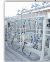
■ Metering pump with manual , electrical and pneumatic stroke adjustment
